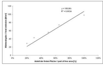
Fig. 4: Heat emission as a function of the free convective area/ the degree of coverage by resting animals (at a temperature difference of 6 Kelvin)
