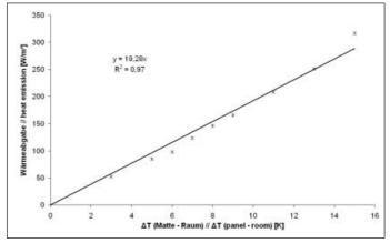
*Fig. 3: In the climate chamber experiment heat emission was clearly a function of the temperature difference between the heating mat and room temperature*
