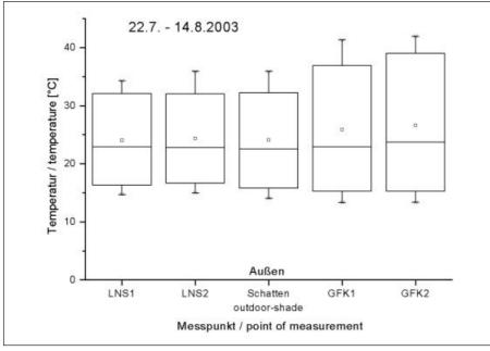
*Fig. 1: Box–whisker-plot of air temperature and shaded outdoor temperature experiment 2 summer 2003*
