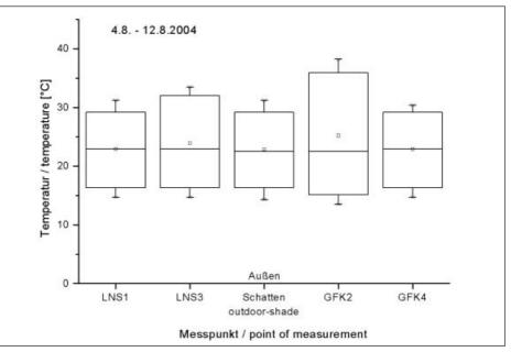
*Fig. 2: Box–whisker-plot of air temperature and shaded outdoor temperature experiment 2 summer 2004*
