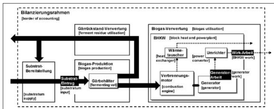
Fig. 1: Scheme of biogas production and energy recovery with selective objects and stock flows
