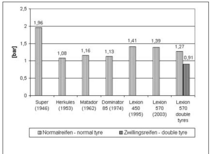
Fig. 2: Average ground contact area pressure at the main axle of the models by full loading calculated by TASC
