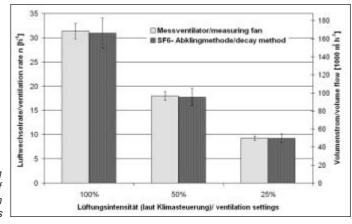
Fig. 2: Comparing measuring methods of different ventilation settings
