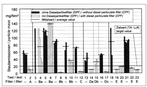
Fig. 1: Particle mass of a rapeseed oil fuelled CHP unit (8 kW<sub>el</sub>) without and with different diesel particulate filters (half-hour average values for exhaust standard conditions, 5 %  $O_2$ )
