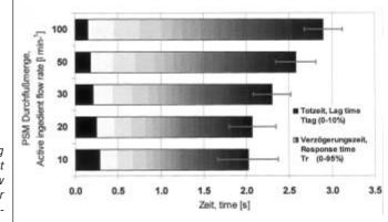
Fig. 1: Comparing lag and response time at constant nozzle flow rate (1.14 l min<sup>-1</sup>) for different active ingredient flow rates
