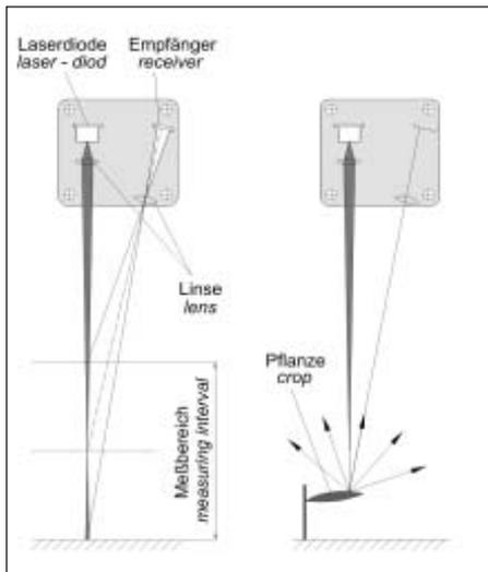
Fig. 1: Measurement principle of laser-triangulation for recording morphological crop
