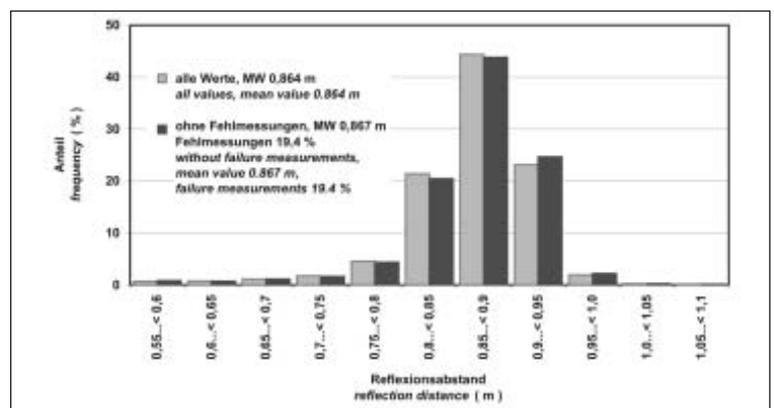
Fig. 2: Frequency distribution of measured data of the sensor LASE ODS 1400 HT
