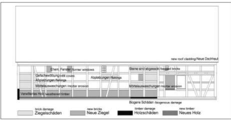
Fig. 1: Surface mapping on a timbered house cladding
