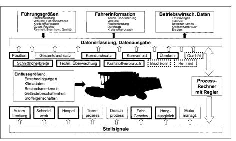
Fig. 1: Control systems on combine harvesters. Bold border: status 2005
