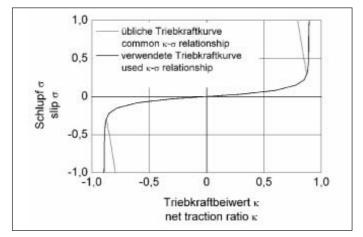
Fig. 1: Common and in the Hohenheim Tyre Model used  $\kappa$ - $\sigma$  relationship
