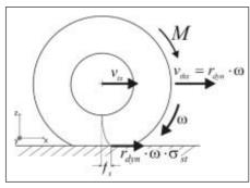
Fig.2: Driven wheel with relevant variables
