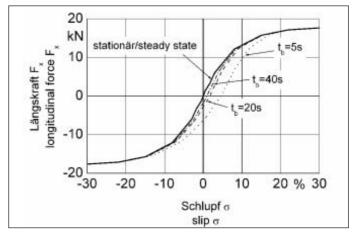
*Fig. 3: Simulated longitudinal forces on a 520/70 R 34 tyre under transient slip conditions*
