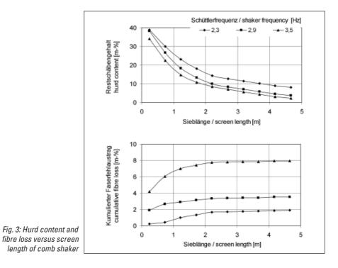
short fibre production. That is why a trial shaker (comb shaker) was developed and tested for detailed study of the structural design under favourable operating and cleaning conditions [7].
