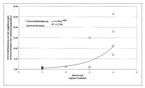
Fig. 2: Ammonia emission from spherically sloped floor and difference degrees of dirtying
