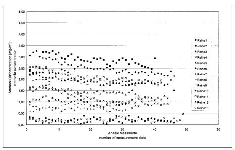
Fig. I: NH<sub>3</sub>-concentration over spherically sloped floors in VS I, measured by wind tunnel method.
