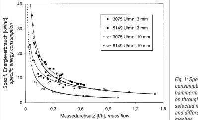
~ 800 kg/m<sup>3</sup>. Average grain diameter derived from three samples was 8.12 mm and in each of the five investigated hammermills the rpm was varied in five steps from 3075 to 5149 min<sup>-1</sup> for each of four to five sieves with  $\emptyset$  from 0.8 to 10 mm and for each rpm step, the throughput was changed, generally in five steps so that in total around 500 measurements were carried out.
