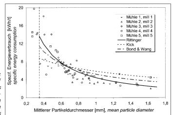
Fig. 2: Minimum specific energy consumption of the hammermills depending on throughput with a range of rpm and final particle diameters
