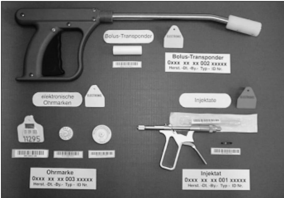
Fig. 1: Transponders used in field (IDEA-Project)
