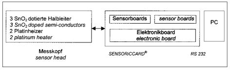
Fig. 2: Schematic view of the Multigas-SENSORiCCARD®.
