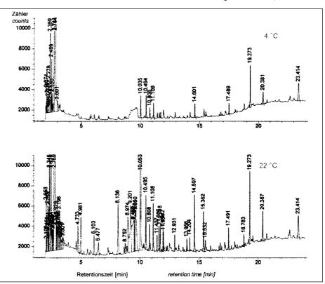
Fig. 4: Headspace analyses of stored apples at 4°C (above) and 22°C (below) recorded by gaschromatography
