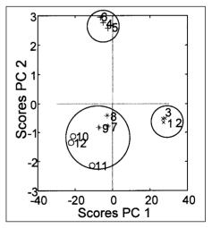
Fig. 3: The PCA of a LIFS (400-580 nm) of mechanical loaded apples (n = 3) during the formation of a brusing damage (1-3= 40, 4-6= 60, 7-9= 135, 10-12= 180 min after impact)
