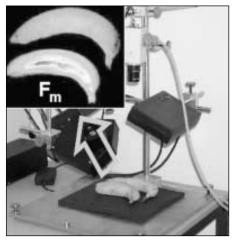
Fig. 2: The chlorophyll fluorescence imaging system FluorCam (Photon Systems Instruments) consists oiLED-panels, habogene saturationpubs lamp, CCV camera and control unit. The very small green parts of the partially ripe banana are easily visible in the lower chlorophyll fluorescence image.
