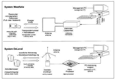
Fig. 1: Principle scheme of electronic activity measurement for dairy cows (systems: Westfalia and DeLaval)
