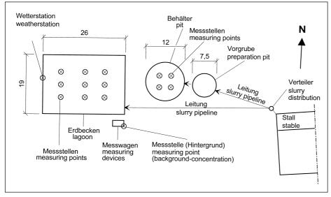
Fig. 1:Slurry pipelines from the stable to lagoon and pit as well as arrangement of measuring points
