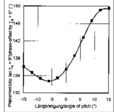
Fig. 8: Angle of pitch influence of phase-offset by cross conveyed angle  $\gamma_q = 0^\circ$
