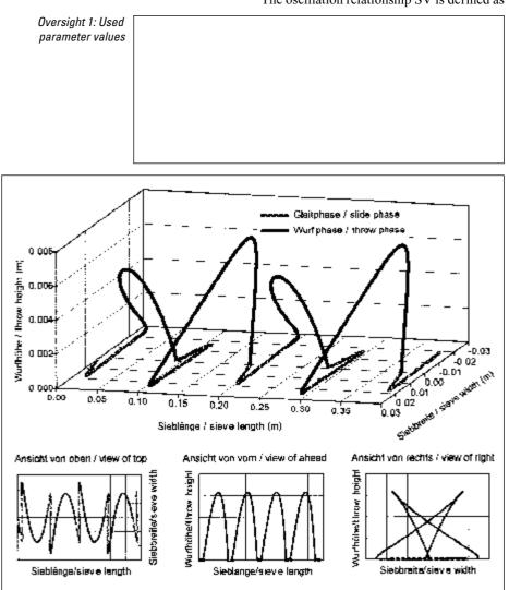
Fig. 2: Motion trajectory relative to sieve with SV = 1.5
