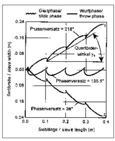
*Fig. 4: Motion trajectories relative to sieve by SV* = 1
