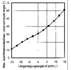
*Fig. 7: Angle of pitch influence of max. cross conveying angle*
