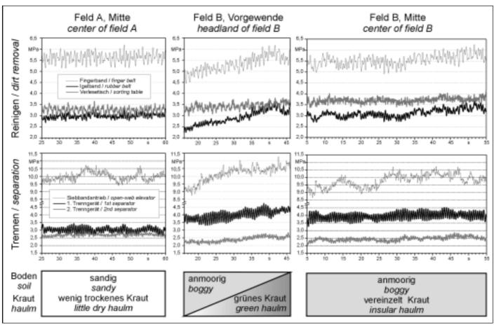
Fig. 2: Pressure readings from separation and dirt removing devices at different operating conditions
