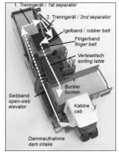
Fig. 1: Potato tracing through the harvester
