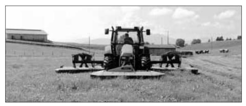
Fig. 1: The mower combination KM5.90 from Deutz-Fahr in "butterfly" mode (two mowers rear, one front-mounted) gives a working width of. 8.50 m.
