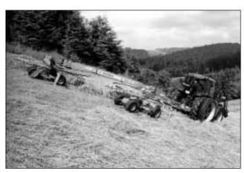
Fig 2: Cardan suspension of the swather-wheels on the Stoll-R 1405 S side windrower allow good adaptability to uneven ground.
