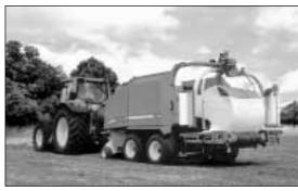
Fig 3: Wrapping of round and big square bales has developed. A number of exhibitors offer improved labour efficiency through combining baling and wrapping in one machine. Here, the John Deere 678 combination baler which avoids the need for separate wrapping operations in the
