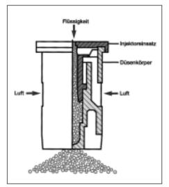
Function diagram of Lechler IDK air injector compact jet
