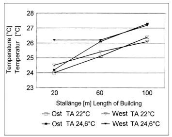
Fig.4: Distribution of temperatures in axial section
