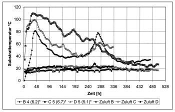
Fig. 2: Course of temperature of inlet air and substrate during composting of pre-dried layer hen droppings, compared with similar aeration rates (\* in [L kg<sup>-1</sup>dry matter<sup>1</sup> h<sup>-1</sup>]) during composting
