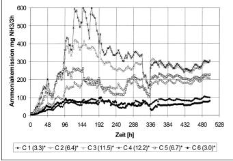
Fig. 4: Course of the ammonia emission released from pre-dried layer hen manure treated with different aeration rates (\*in [L kg<sup>-1</sup>dry matter<sup>1</sup> h<sup>-1</sup>]) during composting
