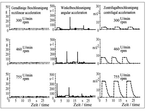
Fig. 3: Acceleration of electronic sugar beet in a lathe at 3 on/off switches
