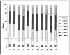
*Fig. 7: Sieve fraction of test run (circular openings: 2 - 67 mm)*
