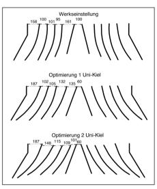
*Fig. 5: Entrance slits (mm) between guiding plates of the chopper with 6.3 m working width*
