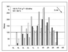
*Fig. 3: Insufficient lateral distribution at 6.1 m working width (11 recording points, 0 in the middle of combine, 4 repetitions)*
