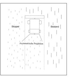
Fig. 6: Unsymmetrical projection by the guiding plates
