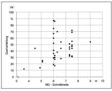
Fig. 4: Lateral distribution and the working width of the combine
