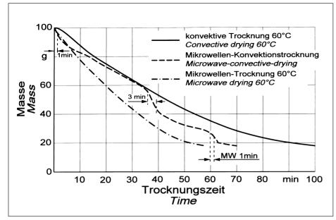
Fig. 2: Drying behaviour of apple slices (3 mm)
