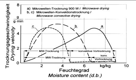
rs - Fig. 1: Drying behaviour of carrot slices (1.5 mm) by microwave drying and microwave drying with tm. convective pre-drying
