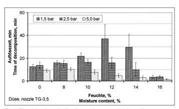
Fig. 4: Dissolving time of soil pellets under a water jet depending on moisture content and water pressure (nozzle TG-3,5)
