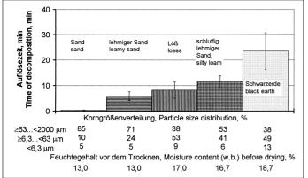
Dried soil pellets from silty-loam sand which had been re-moistened 24 h before the dissolving trials were particularly difficult to dissolve when they had a moisture content of between 12 and 14% (*Fig. 4*). The result agreed with the findings regarding water bath dissolution. The dissolution period decreases in-line with increasing water pressure (Fig. 4).
