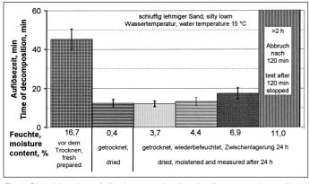
Fig. 3: Dissolving time of silty-loam sand pellets in silent water depending on moisture content
