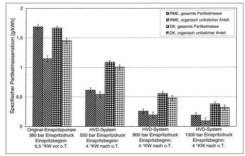
Fig. 1: Specific particulate matter emission of the MWM 302-2 in mode 8 and standard deviation
