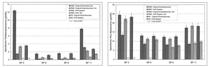
Fig. 2: Measurements in selected modes of the 13-mode test using the original injection pump (injector pressure 380 bar, injection timing 6,5 °ca pre udc) and the HVD system (injector pressure 1000 bar, injection timing 4 °ca after udc) and standard deviation
