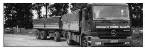
Fig. 2: train with two-axle truck and a three-axle trailer, each tipping construction
