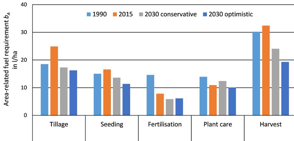
Figure 7: Area-related fuel consumption on the model farm *Fränkische Platte* in the process chain “wheat after rapeseed”
