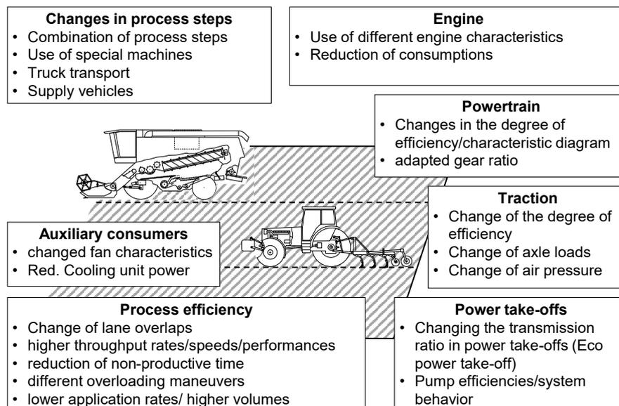
Figure 2: Options for illustrating fuel saving technologies
