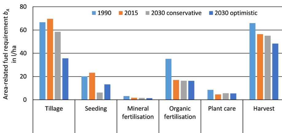
Figure 8: Area-related fuel consumption on the model farm *Southern Bavaria* in the process chain “silage maize after winter wheat”
