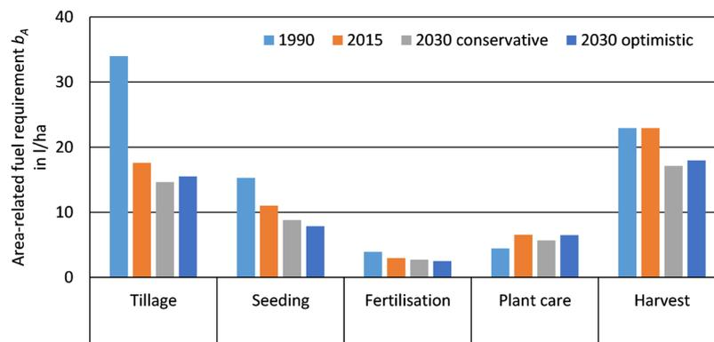
Figure 6: Area-related fuel consumption on the model farm Magdeburger Börde in the process chain “wheat after rapeseed”
