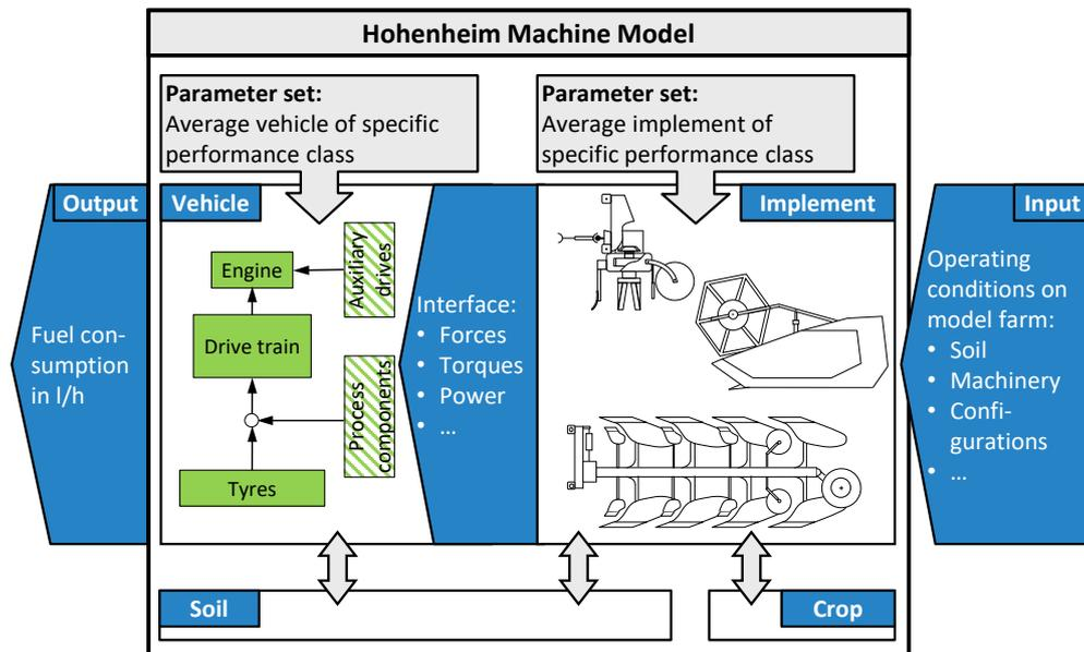
Figure 5: Modular set-up of the Hohenheim Machine Model for the simulation of time-related fuel consumption
