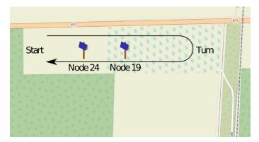
Figure 3: Overview of the test for determining the communication range. The signal strength indicator (RSSI) to nodes 19 and 24 was measured at the two points "Start" and "Turn" on different days. The results are shown in Table 1. (Source of background image: OpenStreetMap)
