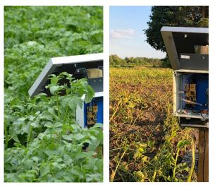
Figure 4: The figures show two different environmental conditions for the collecting nodes on the field. In the first picture the node is almost enclosed by leave of the potatoes, in the second one the node is standing freely in the field.
