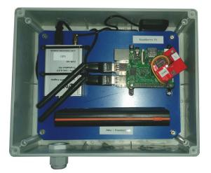
Figure 2: Mobile node on the field sprayer. It contains a GPS, a Raspberry Pi, a rechargeable battery for power supply and a connection for the temperature sensors attached to the sprayer's traverse.
