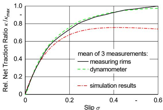
Figure 5: Comparison of net traction ratio between measurement and simulation
