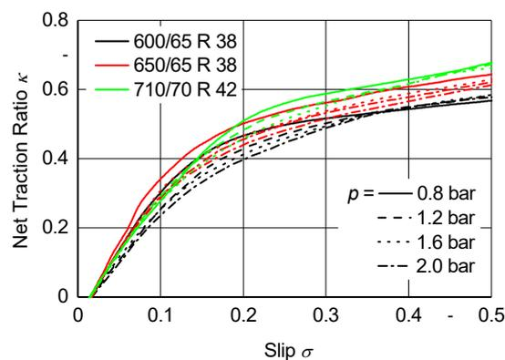
Figure 6: Measured net traction ratio/slip-curves
