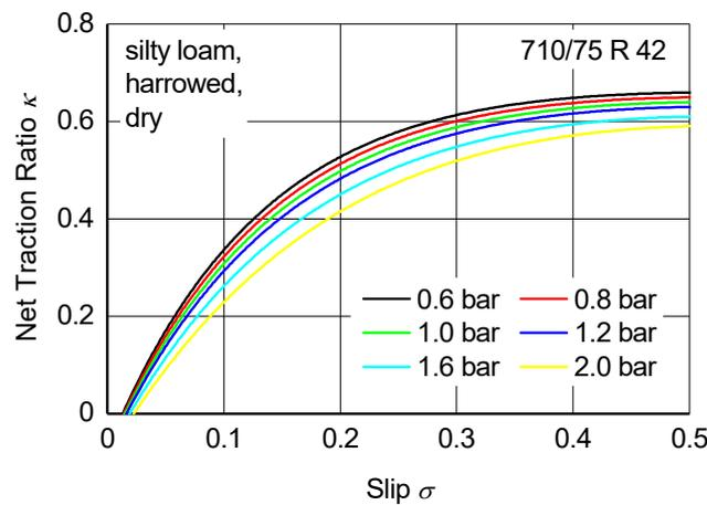
Figure 8: Influence of the tyre inflation pressure when considering the new correction factors
