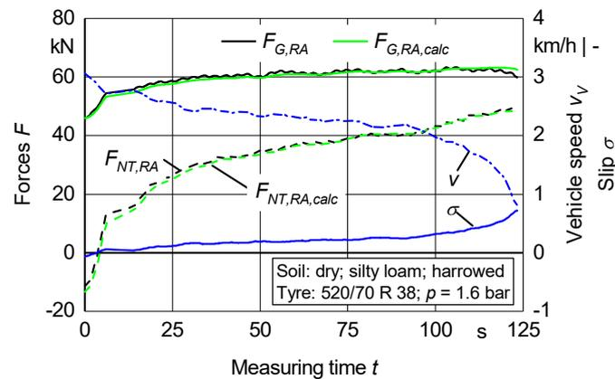
Figure 3: Measured forces, slip and velocity for one test procedure
