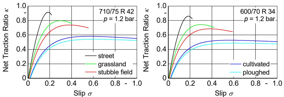
Figure 9: Simulated net traction ratio/slip curves for front and rear wheel of a standard 233 kW tractor in various soil conditions
