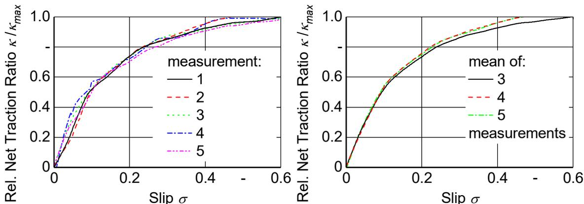
Figure 4: Repeatability of a test
