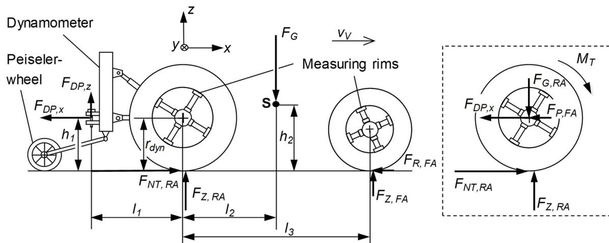
Figure 2: Test setup (left) and resulting forces at the rear wheels (right)
