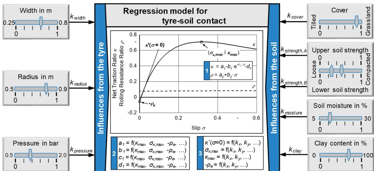
Figure 1: Regression model for the tyre-soil contact
