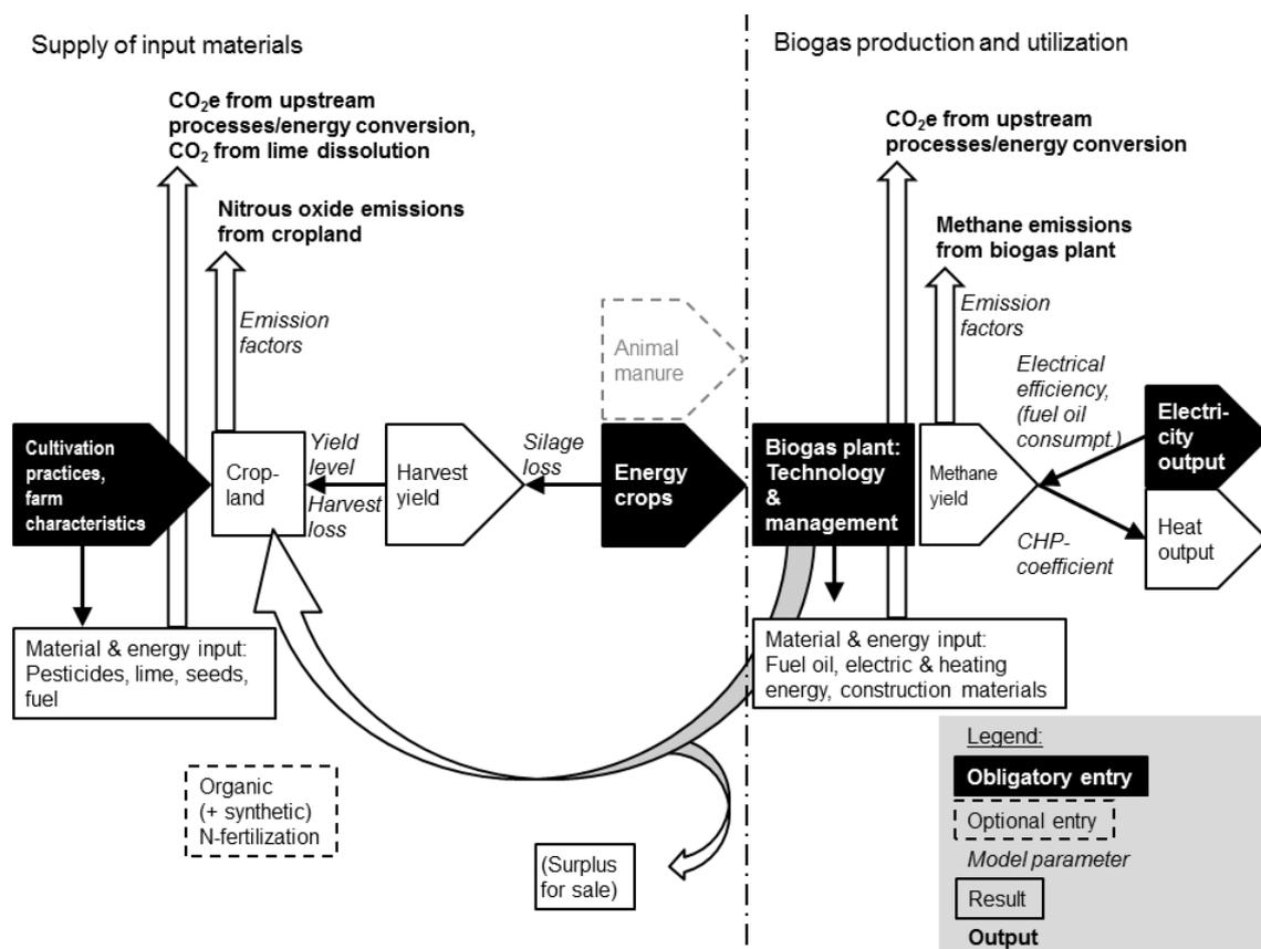
Figure 1: Sketch of the modeled biogas system, reaching from the cultivation of energy crops to the production and utilization of biogas as energy carrier.
