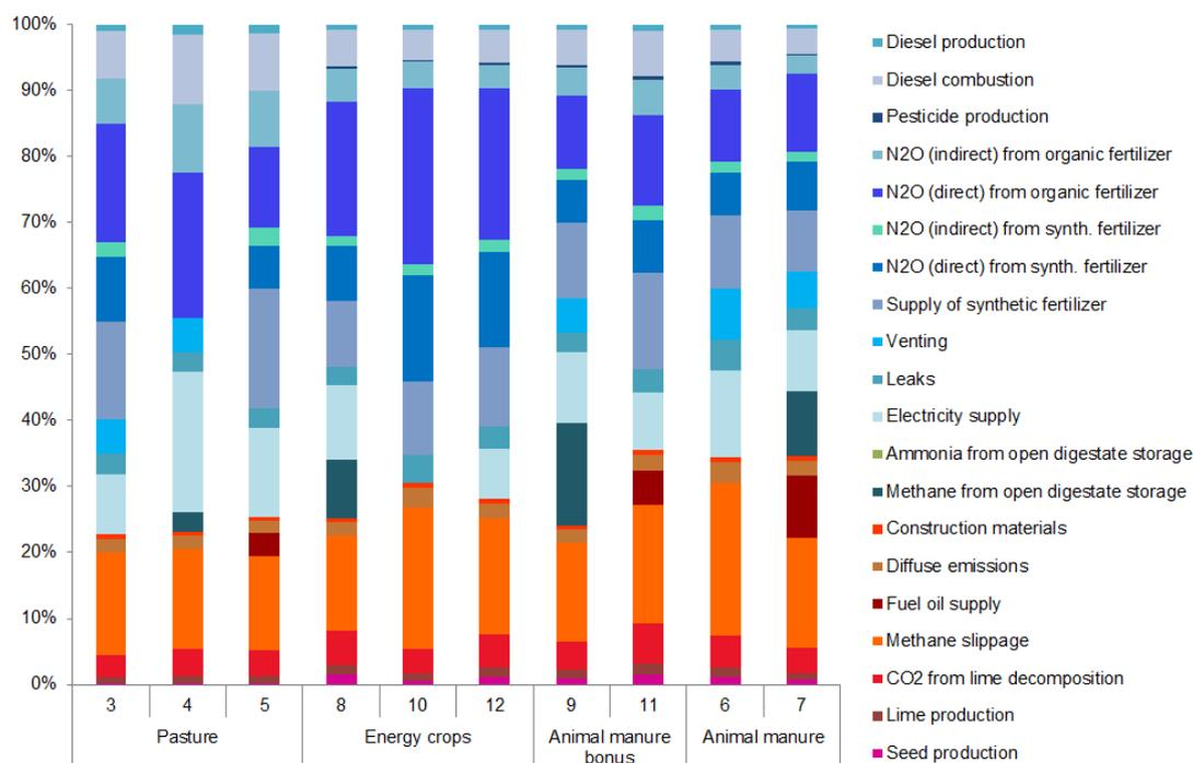
Figure 2: Distribution of specific CO<sub>2</sub>e emissions from individual sources for the ten biogas plants, categorized with respect to input materials.
