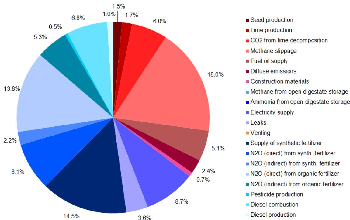
Figure 4: Pie chart from the ‚GHG Calculator‘ web application, illustrating the division of CO<sub>2</sub>e emissions for the biogas process chain of plant „11“.
