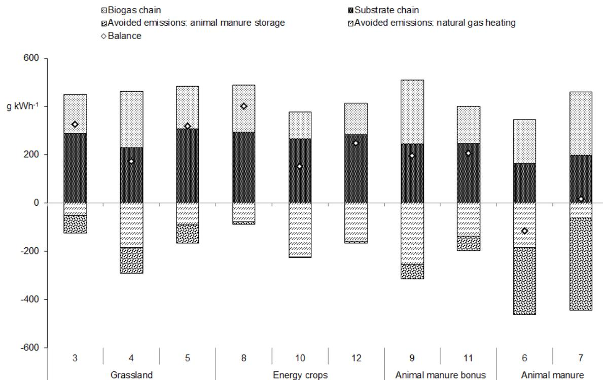
Figure 3: Comparison of the aggregated CO<sub>2</sub>e balance for the provision of electricity, g kWh<sup>-1</sup> for the ten biogas farms, categorized with respect to input materials; calculations were performed using system expansion including avoided emissions from conventional animal manure storage and through substitution of heat from natural gas.
