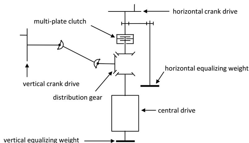
Figure 3: Drive of the sieve of the cleaning unit test rig (MEYER 2015)
