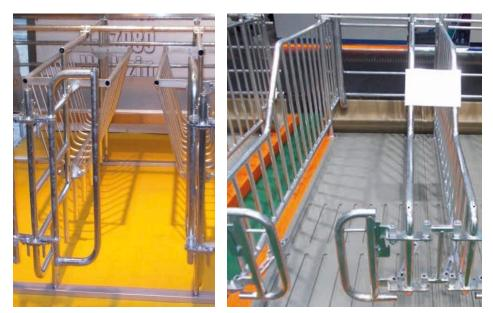
Figure 1: Trapezoid-shaped sow crate and sow crate with a second partition (© S. Meyer-Hamme)
