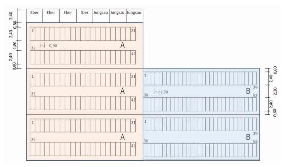
Figure 6: Floor plan of the service area (building 1 and building 2) with sow crates with a width of 90 cm and a length of time of 10 days for small group keeping; 126 animal places in the service area (orange); 116 places in the waiting building with group keeping (blue); scope of stock reduction 10.71 %
