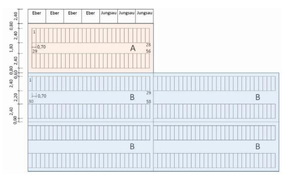
Figure 3: Floor plan of the service area (building 1 and building 2) with sow crates with a width of 70 cm and a stay of 4 days for small group keeping; 56 animal places in the service area (orange); 232 place (4 x 58) in the waiting building with group keeping (blue); scope of stock reduction 3.57 %
