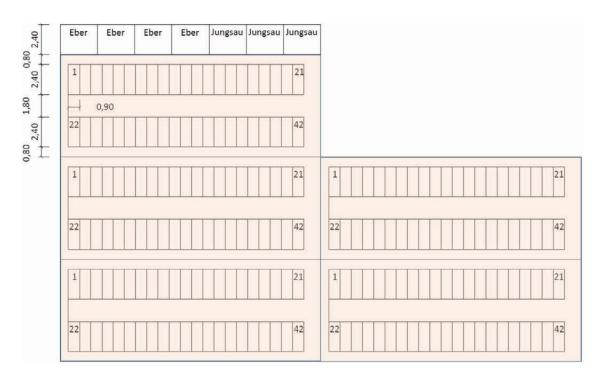
Figure 2: Floor plan of the service area (building 1 and building 2) with sow crates 90 cm apart and 210 instead of the original 280 animal places in 5 compartments with 42 places each (25% stock reduction)
