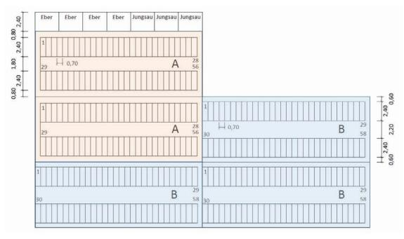
Figure 5: Floor plan of the service area (building 1 and building 2) with sow crates with a width of 70 cm and a length of time of 10 days for small group keeping; 112 animal places in the service area (orange); 174 places in the waiting building with group keeping (blue); scope of stock reduction 3.57 %
