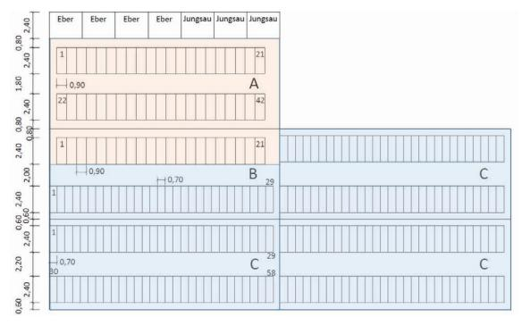
Figure 4: Floor plan of the service area (building 1 and building 2) with sow crates with a width of 90 cm and a length of time of 4 days for small group keeping; 63 animal places in the service area (orange); 203 places in the waiting building with group keeping (blue); scope of stock reduction 7 %
