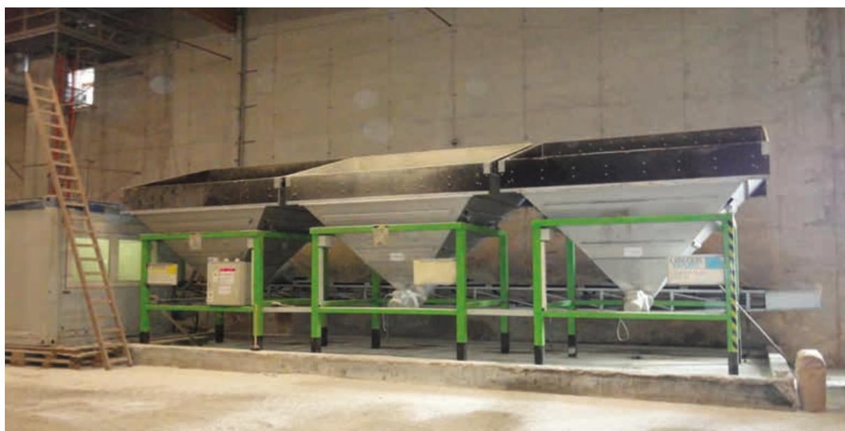
Figure 3: Stationary fertiliser mixing plant, left hopper filled with NPK complex, middle hopper filled with MOP, right hopper filled with CAN (© J. Pichler)
