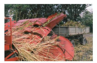
Figure 1: Prototype of a harvesting machine of the IWNIRZ for mowing and separate simultaneous recovery of flowers/panicles (Photo: R. Kaniewski)
