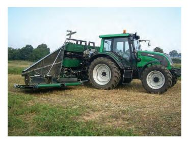
Figure 2: Harvesting machine prototype of the company Kranemann for mowing and and cross-parallel laying of hemp stems (Photo: H.-H. Kranemann)
