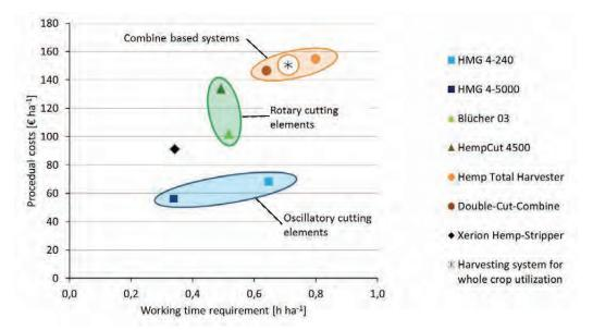
Figure 9: Working time requirement and procedural costs of different harvesting systems (incl. categorized working principles)
