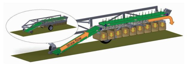
Figure 6: Schematic drawing of a machine for seed gathering from swath deposited hemp crops
