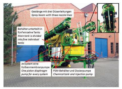
Figure 2: Crop sprayer prototype with direct injection (Photo: M. Krebs)
