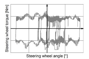
Figure 3: Characteristic of a fully hydraulic steering system
