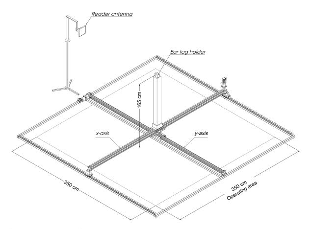
Figure 1: Test bench model diagram
