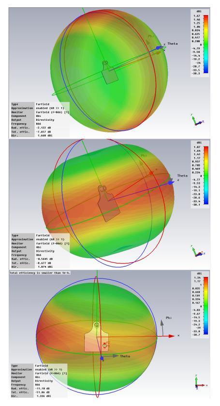
Figure 8: Simulated directional characteristics of ear tags with three basic transponder types (from above: types A and ZT; types B3-4 and B4-4; types C1 and C1-4) (simulation and illustration: deister electronic GmbH, CST Microwave Studio)
