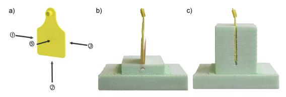
Figure 2: a) Illustration of ear tag orientation to reader (main transmission direction of reader represented by arrows); b) ear tag in "free" positioning (reference variant) in orientation 3; c) ear tag in polystyrene block in orientation 3.
