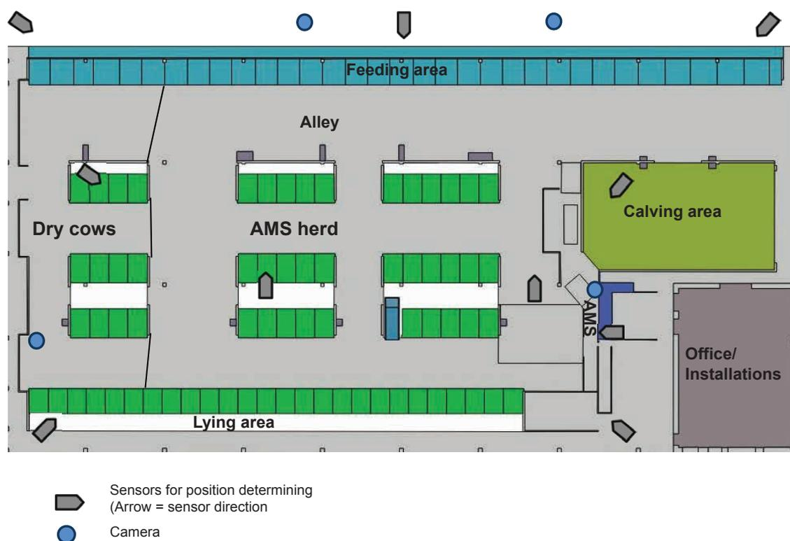
Figure 1: Layout of the freestall barn and positions of recording equipment
