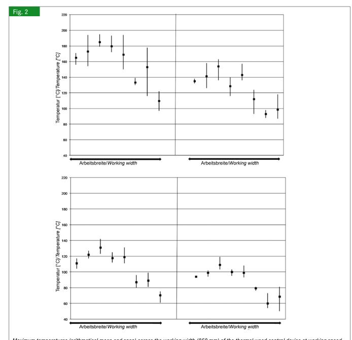
Maximum temperatures (arithmetical mean and span) across the working width (850 mm) of the thermal weed control device at working speed of 0.35 m/s (top left), 0.42 m/s (top right), 0.53 m/s (down left) and 0.81 m/s (down right), (n = 3)
