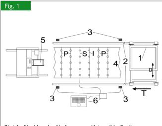
Sketch of test bench with: 1 waggon with top slide, 2 rails, 3 photoelectric relays, 4 target surface with holes for thermocouples (S), model plants (P) and indicators (I), 5 winch, 6 device for data sampling and data storage, T direction of travel, D direction of displacement
