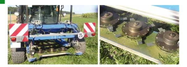
Test machine with functional prototype mower (left) and mower bar with cutting units "2/2" (right) (Photos: S. Kemper)
