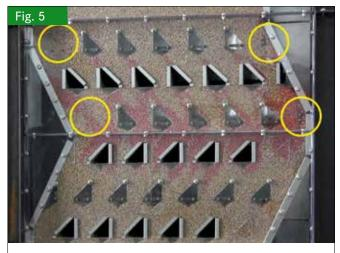
Particle flow profile in the new designed dryer geometry with optimized number of air ducts (Photo: ATB)
