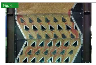
Particle flow profile of colored wheat particles in the test dryer with new design and maximum number of air ducts (Photo: ATB)
