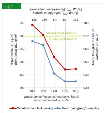
Influence of raw material moisture on physical-mechanical properties and energy input
