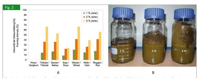
Foaming intensity in digestate from a biogas plant using renewables after addition of 1, 2 and 3 % (w/w) coarse grain and soya (2 mm), respectively, after 22 hours test duration (A); Experiment with rye groats as substrate (B) (Foto: L. Moeller)
