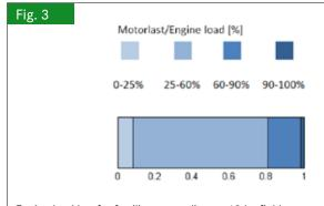
Engine load bar for fertilizer spreading on 10 ha field, tractor power: 261 kW
