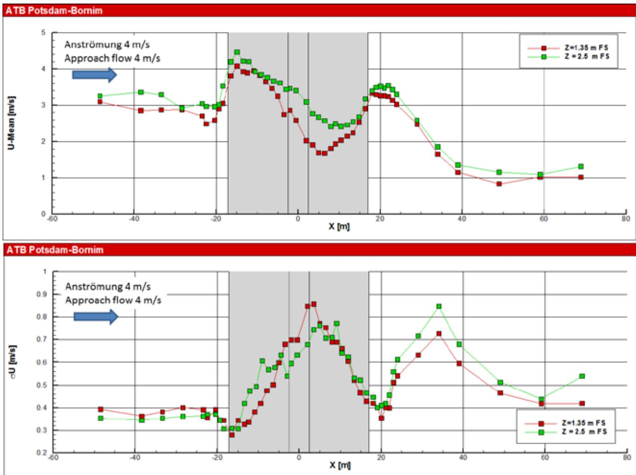
Measured profiles of the mean wind component  $U$  in  $x$ -direction (above) and the standard deviation  $\sigma_U$  (below). Grey area indicates area of the barn including feeding alley in the center.
